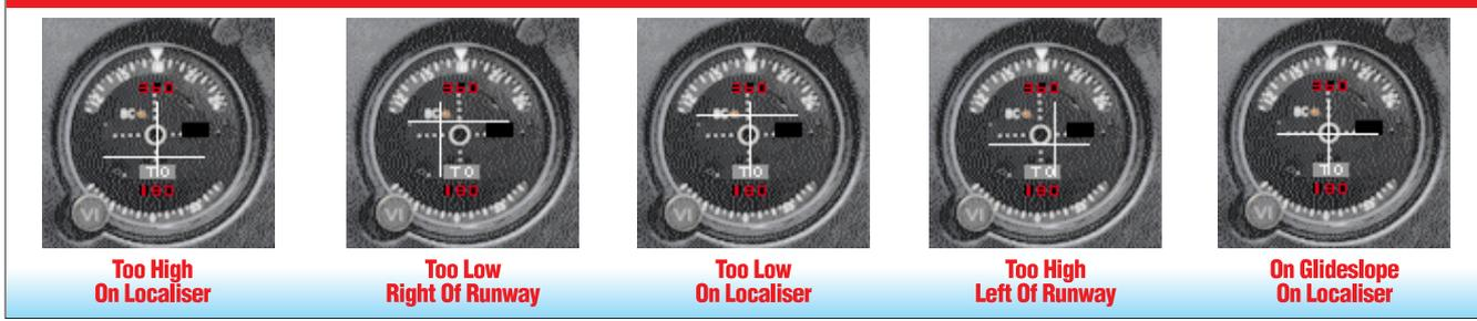
Above: The ILS receiver in the aircraft. The vertical needle is the localiser, the horizontal needle is the glideslope. The circle in the centre is your aircraft. The aim is to centre the needles in the circle as illustrated on the far right.
