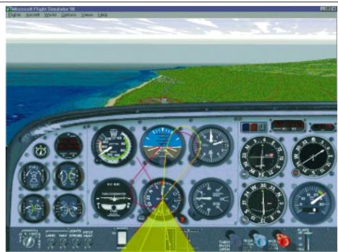
Once established at 2,000 feet, turn left onto  $055^\circ$ . You will find the OBI needle is more or less centred when you roll out. Make small adjustments to either your heading to re-intercept, or the OBS to centre the needle.
