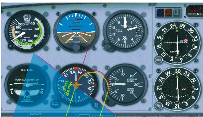
We are definitely in Sector 3. This can be determined by noting the imaginary line at  $70^\circ$  to the inbound. This line would be  $(270^\circ \text{ inbound} - 70^\circ) 200^\circ$  through  $020^\circ$ .
