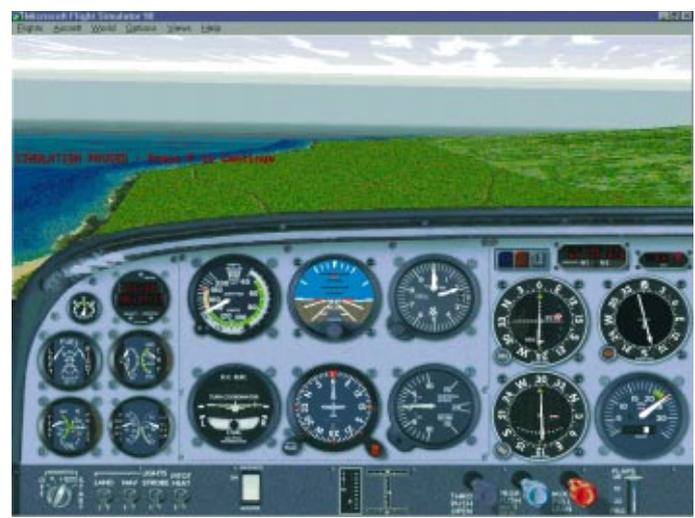
Established outbound in the teardrop. Time will be up at 08:17:20 (3 seconds from now). I then turn onto  $270^\circ$  and set  $270^\circ$  on the OBS during the turn.
