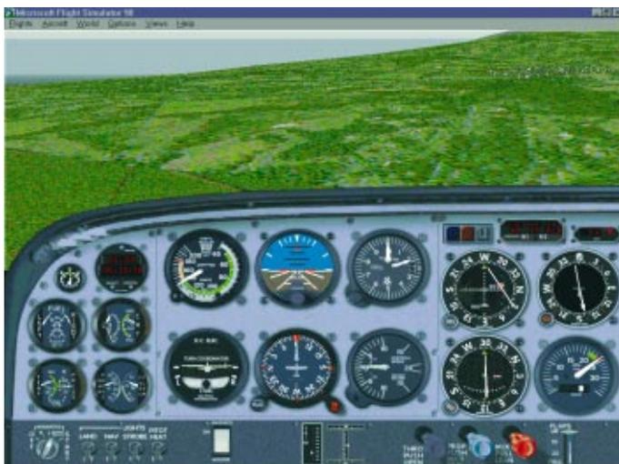
Established on the parallel leg with 270° set up on the OBS in preparation for the inbound intercept. I am waiting for the time (8:15:40) before I begin a turn all the way left to pick up the inbound leg.
