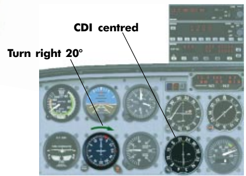
Aircraft at 12.5 DME. Require 20° heading Change to correct
