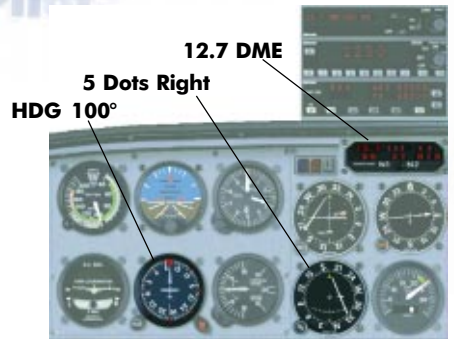
Display after initially turning to 100° and holding HDG until CDI bar fully to right (5 dots), DME 12.7 - begin turn to right
