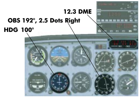
Heading=100°, OBS=192°, CDI=2.5 dots right, DME=12.3, Altitude=3000ft
