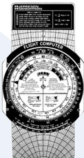
**One example of a pilot's flight computer. Smaller versions are available that fit in your shirt pocket.**
