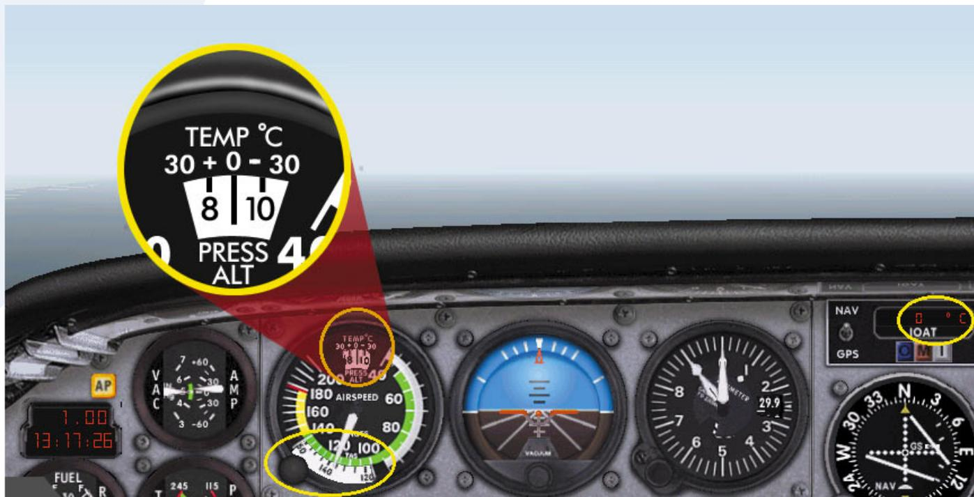
Reading TAS directly on the ASI by setting 9000 feet against the outside air temp of 0°C.
