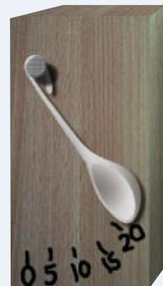
The density of water is abundantly greater than the conditions used during the calibration: The spoon ASI over reads.
