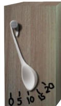
Airspeed Indicator Mark I - The airflow moves the spoon allowing you to read off air speed.
