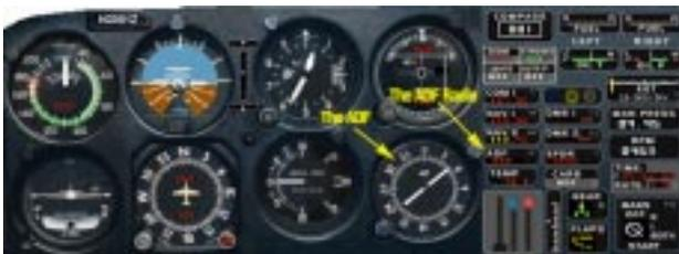
The ADF on the Flight Simulator instrument panel
